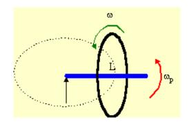
The wheel is a rotating object so its angular momentum is given by I $\Omega$ . Treating the wheel as a hoop, I =  $mr^2$ . Thus
