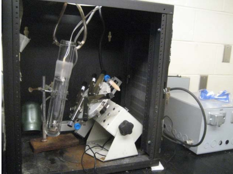
Figure 2.4 Experimental set up for perchlorate reduction using zero valent iron without UV light.
