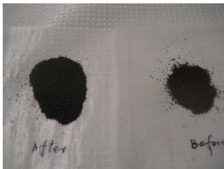
Figure 2.2 Image of iron filings before and after HF washing.
