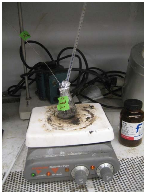
Figure 2.1 HF washed iron filing drying set up.
